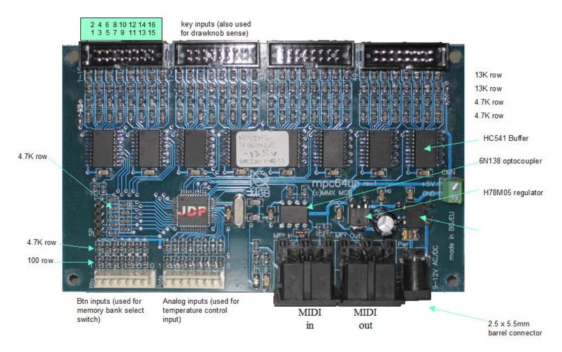
Encoder sn001 has the 13K input resistors. Encoders 2,3,4 have 8.2K input resistors due to a misunderstanding when they were ordered. The mpc64up-usman.pdf user manual is include in the appendix.
